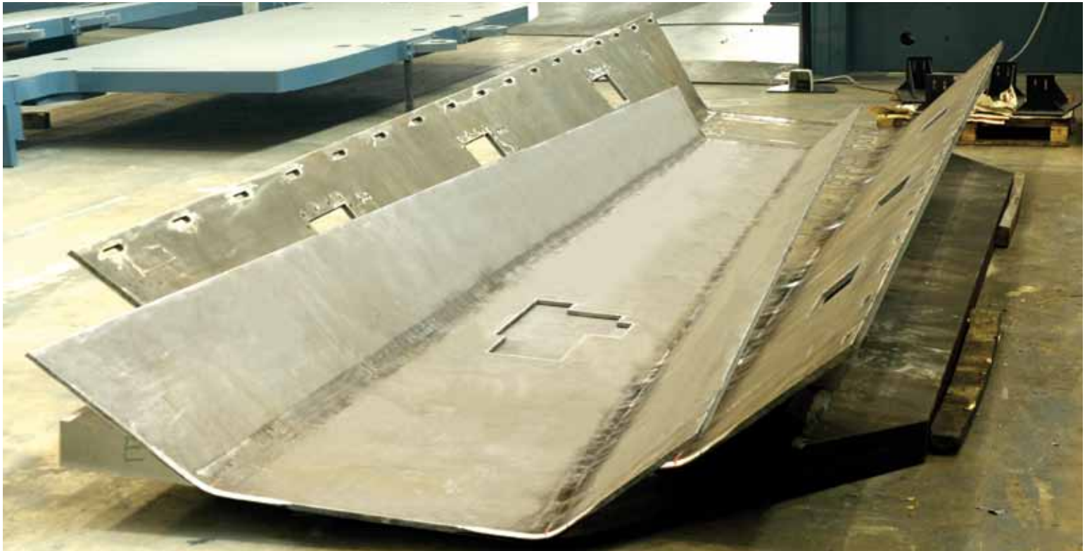
3/4" Thick Special Steel Armox for Defense Industry
